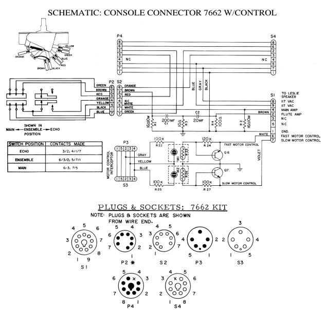
\* WIRE P2 ACCORDING TO DRAWING. DO NOT WIRE ACCORDING TO EMBOSSED NUMBERING ON REAR OF PLUG. Page  $2\ {
