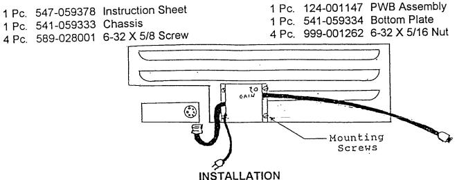
The easiest installation method is to plug in the 6 foot, 11 conductor cable to the 11 pin-socket on the rear of your organ or keyboard, then plug the short 6 conductor cable directly into the 147 or into the 30' cable that was supplied with your 147. Now connect the power cord from the 1147 Kit to a source of 220 Volt 60 Hz power.
