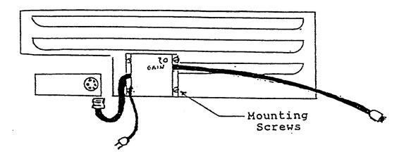
The easiest installation method is to plug in the 6-foot 11-conductor cable into the 11-pin socket on the rear of your organ or keyboard, then plug the short 6-conductor cable directly into the Leslie Speaker cabinet or into the 30' cable that was supplied with your cabinet. After this is done, connect the AC power cord from the 1122 Kit to one of the following power sources (see label):
