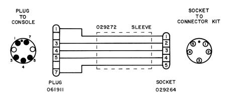
NOTE: DRILL OUT PINS 2 & 6 ON PLUG, 061911
